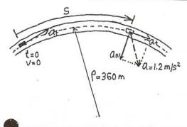
The train starts from rest at t = 0 (s = 0). The tangential acceleration  $a_t$  remains constant whereas  $a_n$  slowly increases as v increases. When the speed reaches 70 km/h (19.44 m/s)  $a_n = (19.44)^2/360 = 1.05 \text{ m/s}^2$
