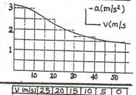
Since (1/a) dv = dt, if a curve of 1/a versus v is plotted and the area under the curve is taken from v = 25 m/s (or 90 km/h) to v = 0 we directly get time required to stop.
