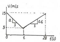
Prob.: The maximum possible deceleration of a passenger train under emergency conditions was determined experimentally, the results are shown (solid curve) in the figure. If the brakes are applied when the train is traveling at 90 km/h, determine by approximate means (a) the time required for the train to come to rest, (b) the distance traveled in that time.
