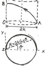
We know that  $a_t = \overline{e}_t$ .  $\overline{a}$  where  $a_t$  is the tangential acceleration component and  $\overline{e}_t$  is a unit vector in the tangential direction. e, is found by dividing the velocity vector by its magnitude Thus
