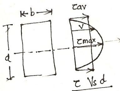
NOTE : See FM : similar to velocity distribution diagram of a channel section in which velocity distribut<sup>n</sup> is parabolic & max. vel. is at midpoint where as avg. vel. is assumed as shown.
