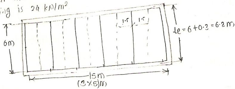
① Each beam will carry load of 3m wide slab.
