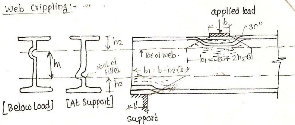
$$\text{Bearing stress } \delta p_{cal} = \frac{P}{\text{Bearing area pro.}} = \frac{P}{b_1 \cdot t_w}$$
