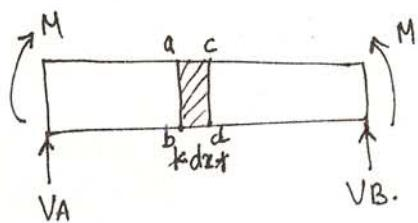
Pure Bending / simple bending
