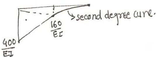
$$\Delta C = \frac{400}{EI} \times 0.5 \times 3 [4 + 2] + \frac{160}{EI} \times 0.5 \times 3 [4 + 1] + \frac{1}{3} \times \frac{160}{EI} \times 4 \left[ \frac{3}{4} (4) \right]$$
