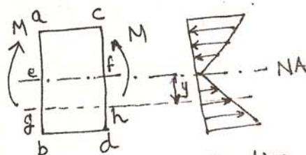
FBD of strip 'abcd'. Bending stress diagram.
