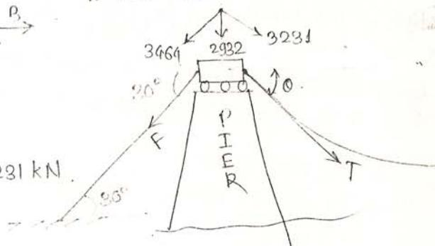
$$\begin{aligned} &\text{: Eqm condition,} \\ &F \cos 30 = T \cos (21.8) \\ &\therefore F = 3231 \frac{\cos(21.8)}{\cos 30} \\ &\boxed{F = 3464 \text{ kN}} \end{aligned}$$
