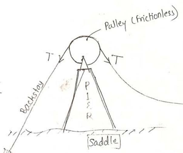
Ques:- Find the tension in the backstay & the pre. on the pier, if the cable is saddle & the backstay is at  $30^\circ$  with the horizontal.
