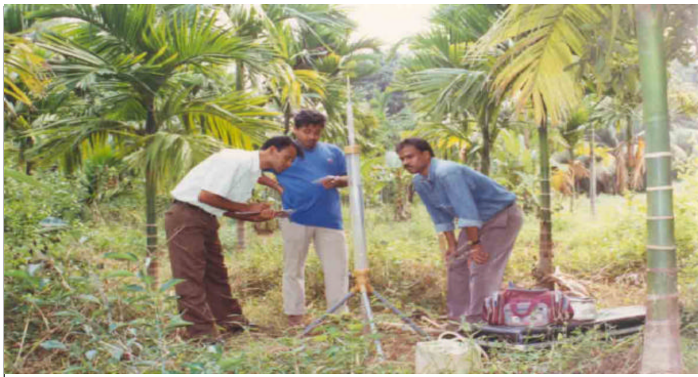
Infiltration study with Guelph permeameter in a watershed near Guwahati, Assam
